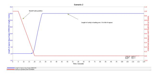
In this scenario the shutoff valve closes, the loading pump stops, the bypass valve opens and the cargo tank has a back pressure of 2.5 barg.
