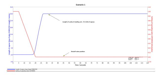
In this scenario the shutoff valve closes, the loading pump stops and the bypass valve opens.
