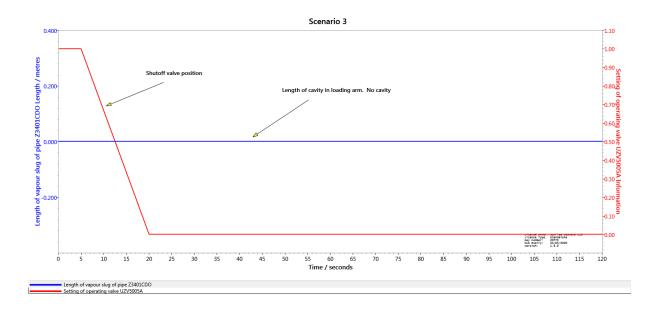
In this scenario the shutoff valve closes, the loading pump stops, the bypass valve opens, the cargo tank has a back pressure of 2.5 barg and the tank valve closes.
