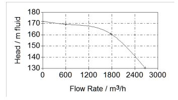
3.2. One of the two aft pumps starts at 5 secs and runs up in 7 secs. The inlet pressure of the pump is constant at 0.55 barg.
