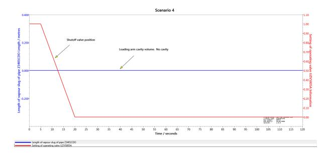
In this scenario the shutoff valve closes, the loading pump stops, the bypass valve opens, the cargo tank has a back pressure of 2.5 barg, the tank valve closes and the apex of the loading arm is increased to 46.5 m above the shutoff valve.
