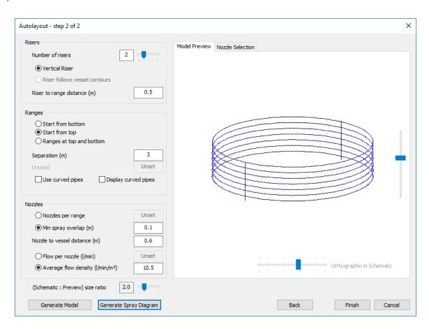
Once the model has been generated, you can check the corresponding calculated nozzle data in the Nozzle tab:
